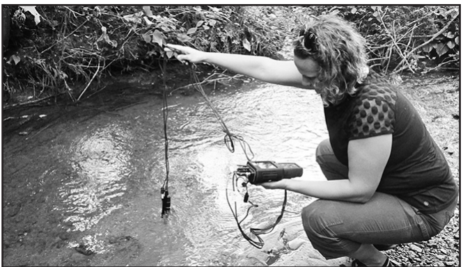
HRWC volunteer monitoring program coordinator, Amanda Kanack uses a meter to measure dissolved oxygen, pH and other water quality parameters from a local stream.
